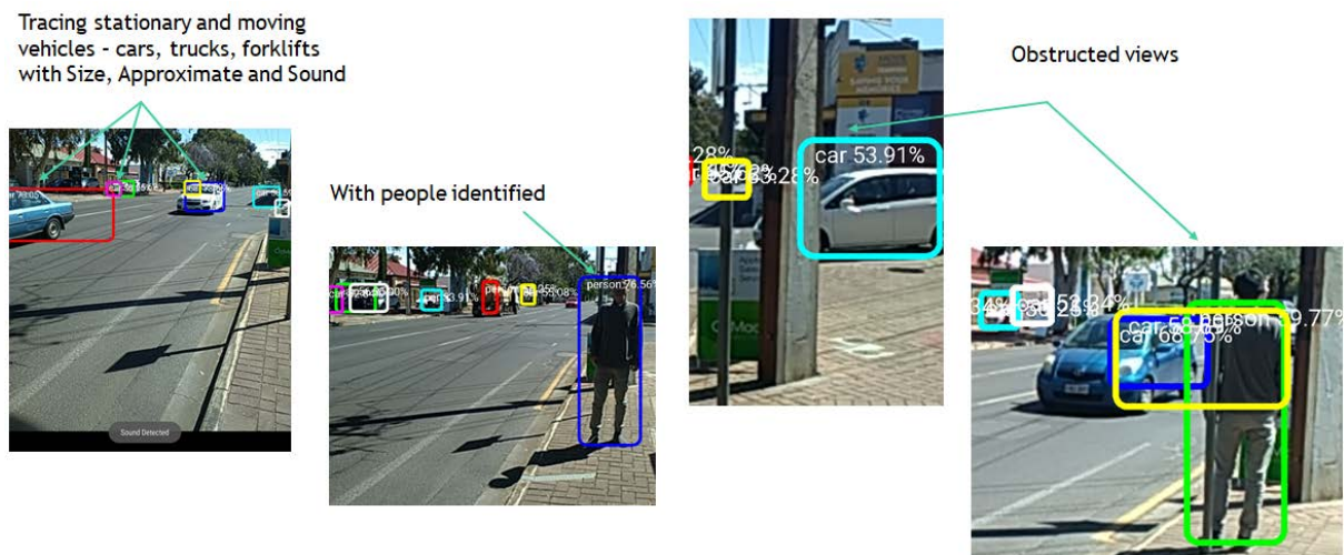
Figure 3: Initial experimental trial to demonstrate the object detection ability with % accuracy in the display
