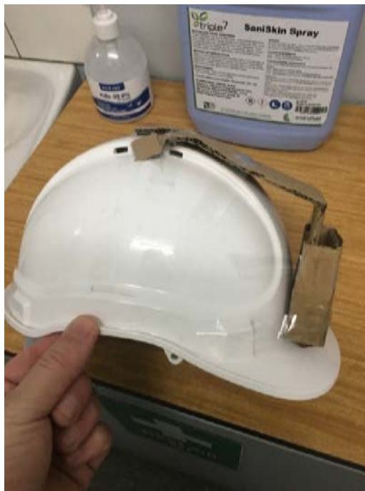
Figure 1: DIY helmet mounted system (Smart Phone in use) – camera focusing set to 1 to 50 meters
