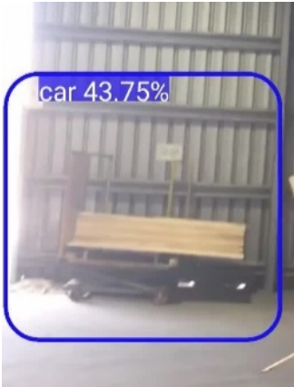
Figure 5: Error – A mobile trolley is recognised as a vehicle
