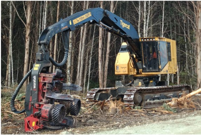
Figure 4: A Tigercat LH22D harvester with Waratah HTH622B harvesting head and a Ponsse Elephant King forwarder were used at the Unpruned Low-Quality (ULQ) and Pruned High-Quality (PHQ) sites.
