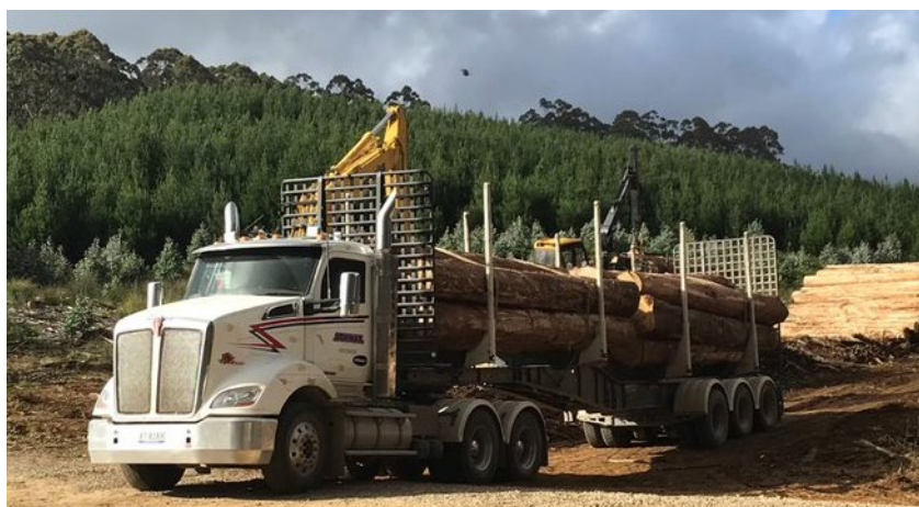
Figure 6: A Komatsu 270 log loader loading a truck and 2-bunk trailer at the Pruned High-Quality (PHQ) site.
