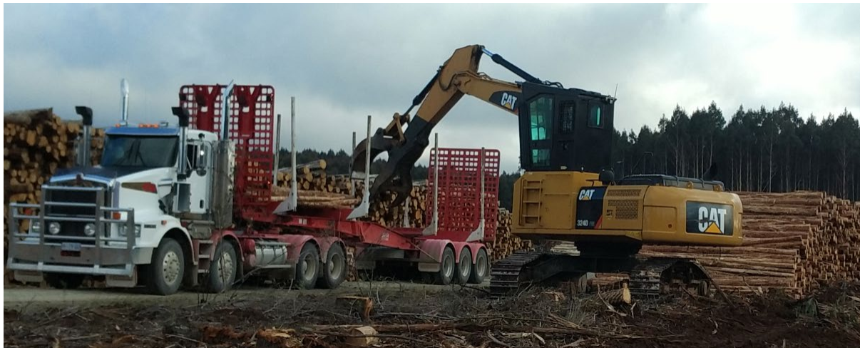
Figure 5: A Caterpillar 324D log loader loading a truck and 2-bunk trailer at the Unpruned Low-Quality (UHQ) site.
