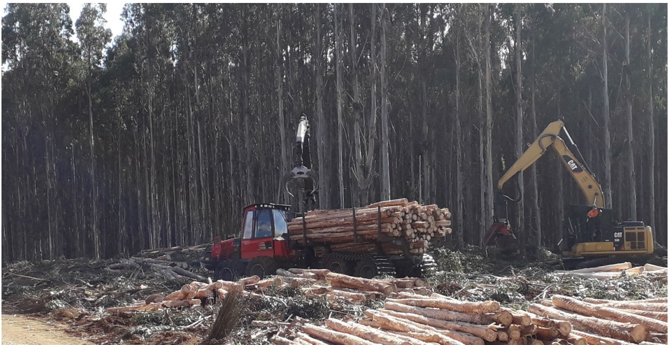
Figure 3: A Komatsu 895 forwarder and a Caterpillar 538 excavator with Waratah HTH622B harvesting head were used at the Unpruned High-Quality (UHQ) site.
