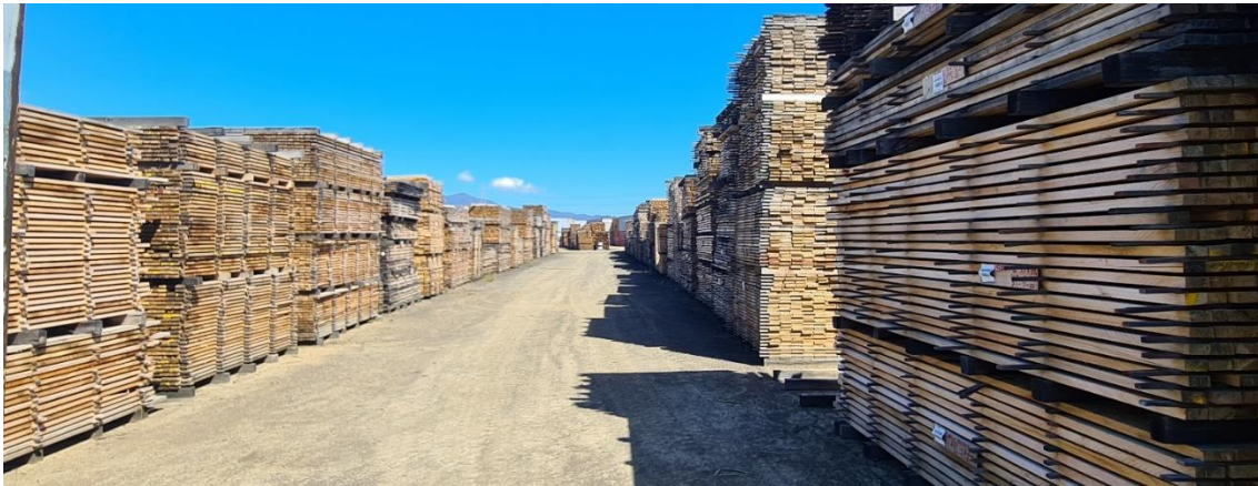
Figure 1: Conventional hardwood drying yard: line stacked
