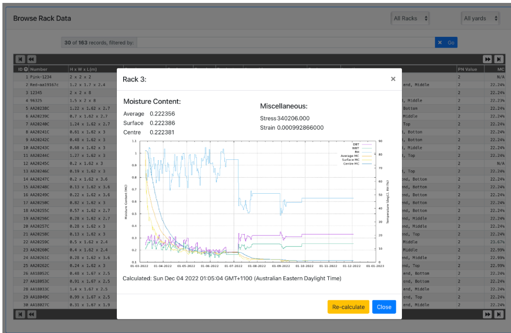
Figure 31: HI AirDry app: Drying estimate for a single rack.
