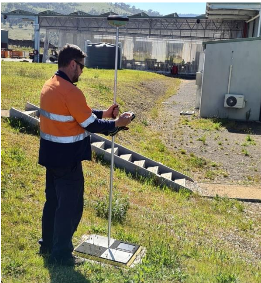
Figure 3: Confirming the position of GPS plates
