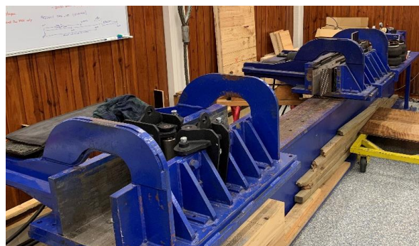
Figure 29. Custom designed and built rolling compression set up. Photo: Rhianna Robinson.
