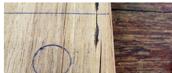
Figure 47. Irreversible damage following densification of Tasmanian oak. Photo: Benoit Belleville.
