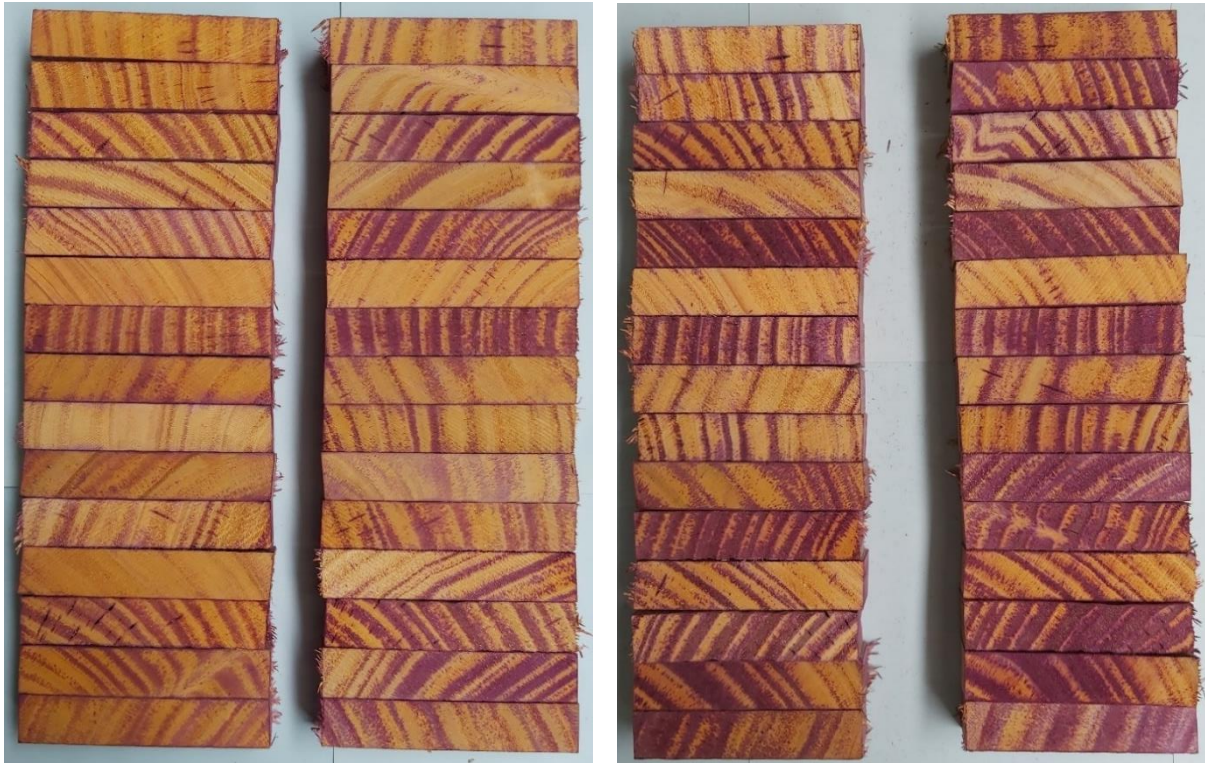
Figure 13. Penetration images of treated shining gum from charge 3+MCA+adjuvants, left to right, showing copper penetration of MCA, MCA + B, MCA + S and MCA + V. Photo: Stuart Meldrum.
