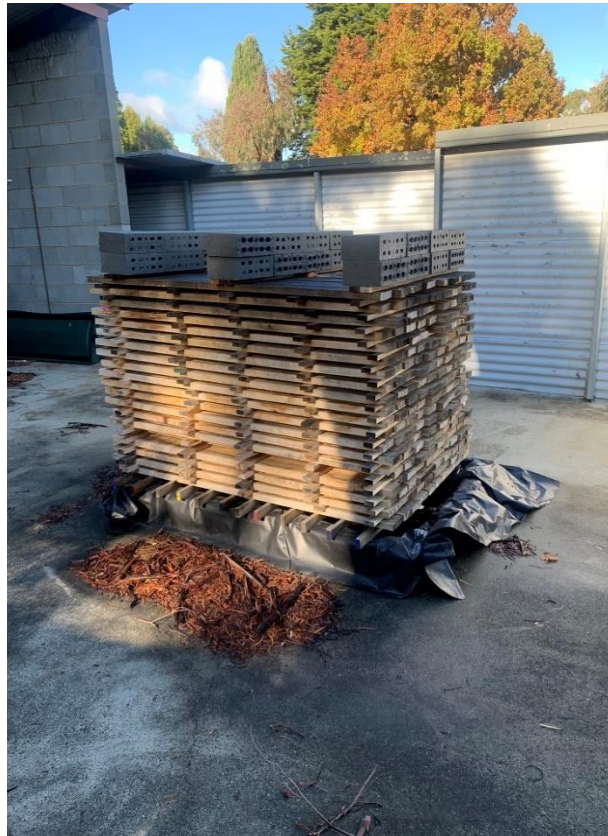
Figure 6. Unsheltered rack of boron treated shining gum boards air drying at T40, with leachate collection set up underneath. Photo: Kyra Wood.
