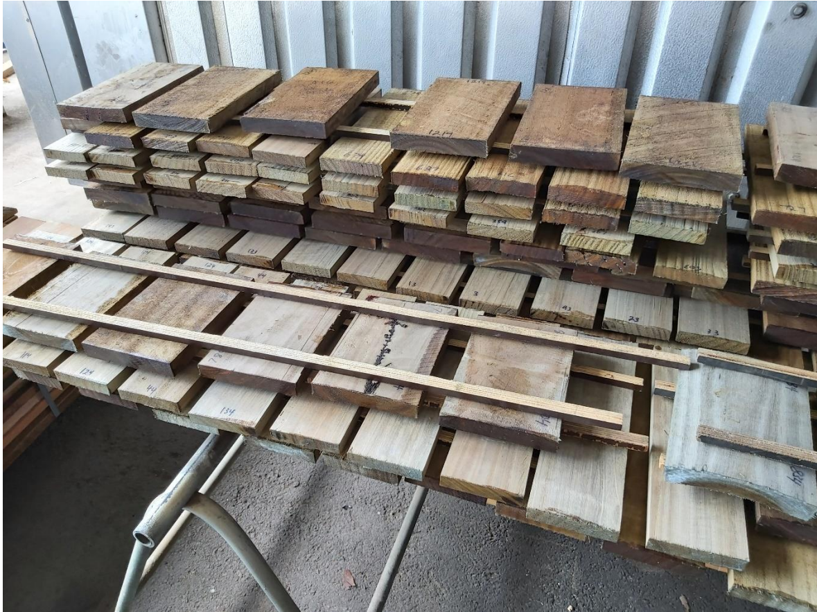
Figure 11. Samples air-drying following treatment. Photo: Rhianna Robinson.
