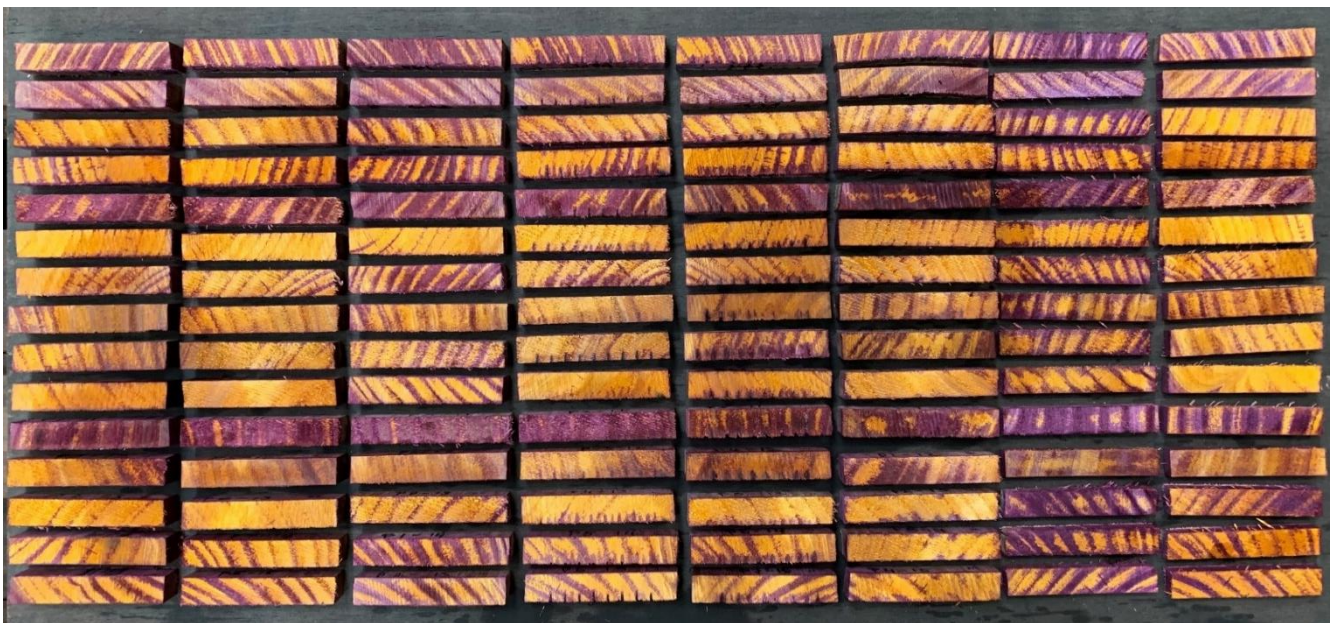
Figure 31. Pre-treatment comparison penetration images for shining gum samples treated with charge 1 + MCA + V. Photo: Rhianna Robinson.
