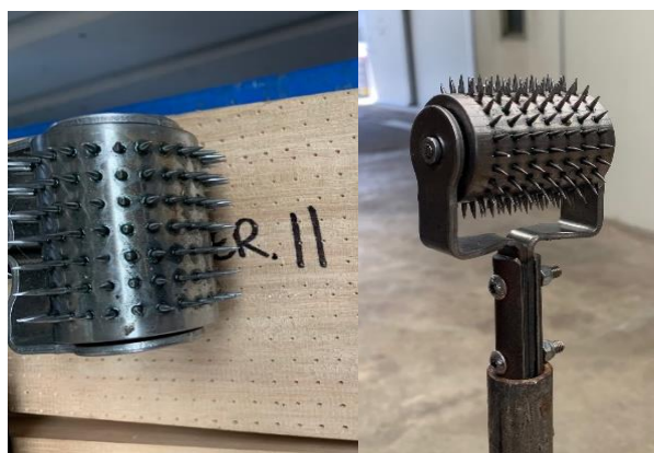
Figure 20. Spiked roller incision set-up. Photo: Rhianna Robinson.
