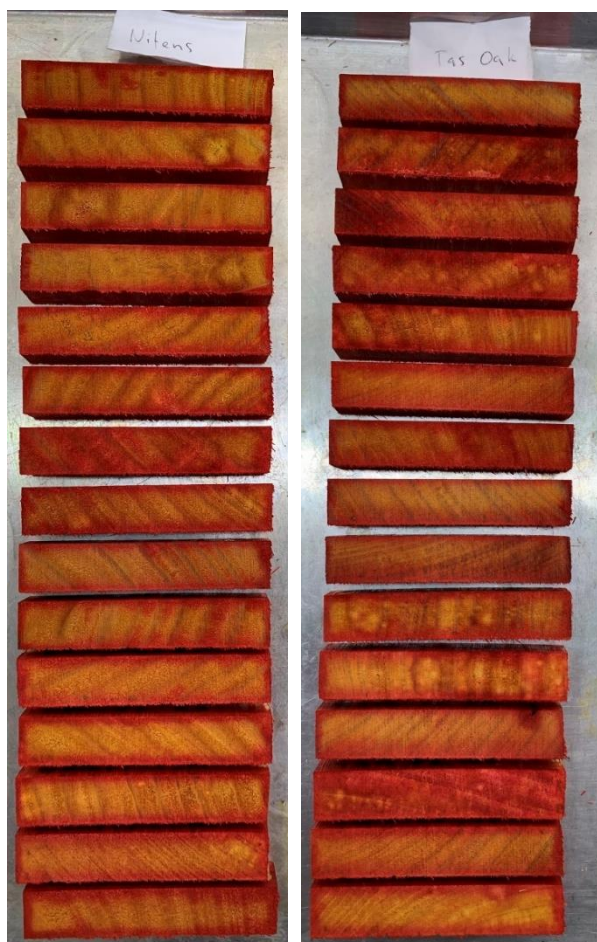
Figure 37. Penetration images for Kop-Coat 'best bet' trial samples sprayed with boron-reactive indicator spray (RHS shining gum; LHS Tasmanian oak). Photo: Rhianna Robinson.
