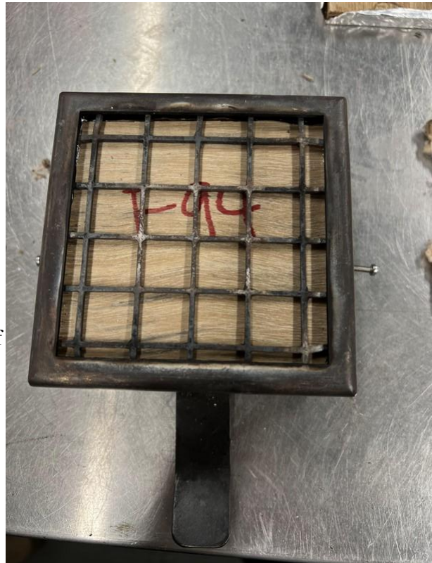
Figure 55. Grid used to prevent sample from delaminating during cone calorimeter test. Photo: Wenxuan Wu.
