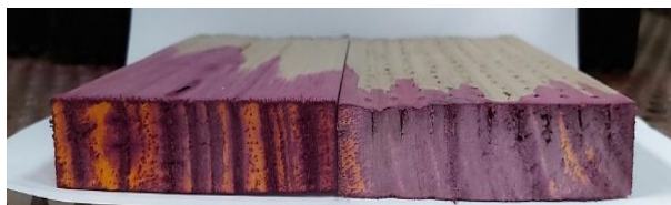
Figure 23. Penetration images of laser incision patterns following treatment. Photo: Rhianna Robinson.
