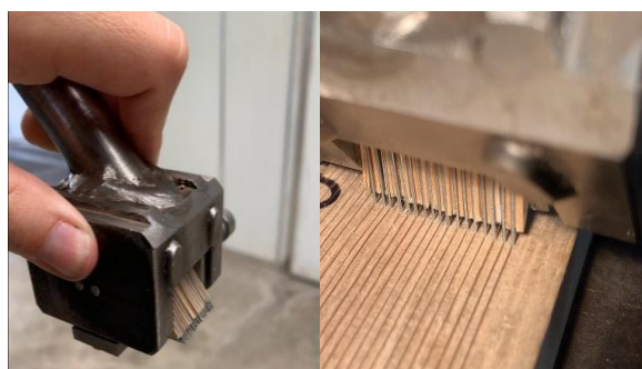
Figure 18. Blade incision set-up. Photo: Rhianna Robinson.
