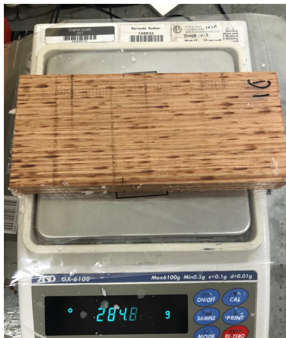
Figure 2. Samples being weighed after dipping. Photo: Ros Ghani
