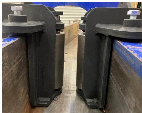
Figure 28. Custom designed and built rolling compression set up. Photo: Rhianna Robinson.
