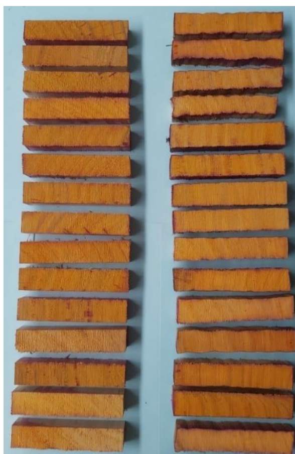
Figure 14. Penetration images of LOSP treated shining gum (LHS seasoned), (RHS GOS). Photo: Stuart Meldrum.
