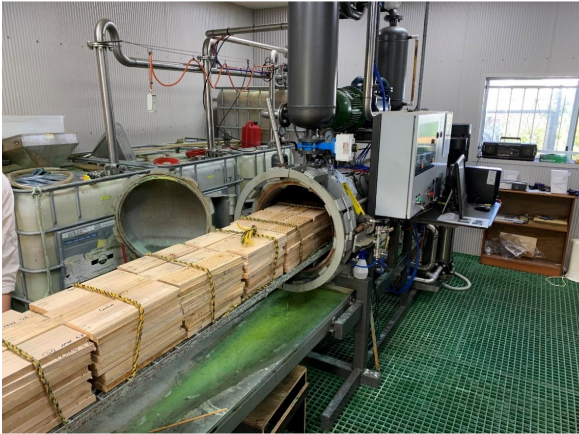
Figure 9. Samples awaiting treatment in the VPI cylinder at the Salisbury Research Facility. Photo: Rhianna Robinson.
