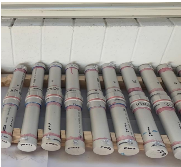
Figure 4. Diffusion cup apparatus. Photo: Kyra Wood.
