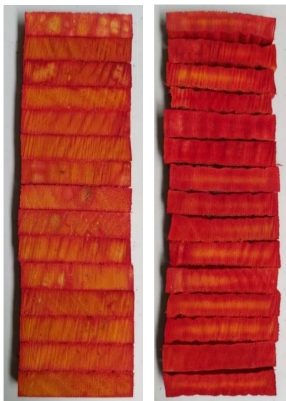
Figure 15. Penetration images of Kop-Coat treated shining gum (LHS seasoned; RHS GOS). Photo: Rhianna Robinson.
