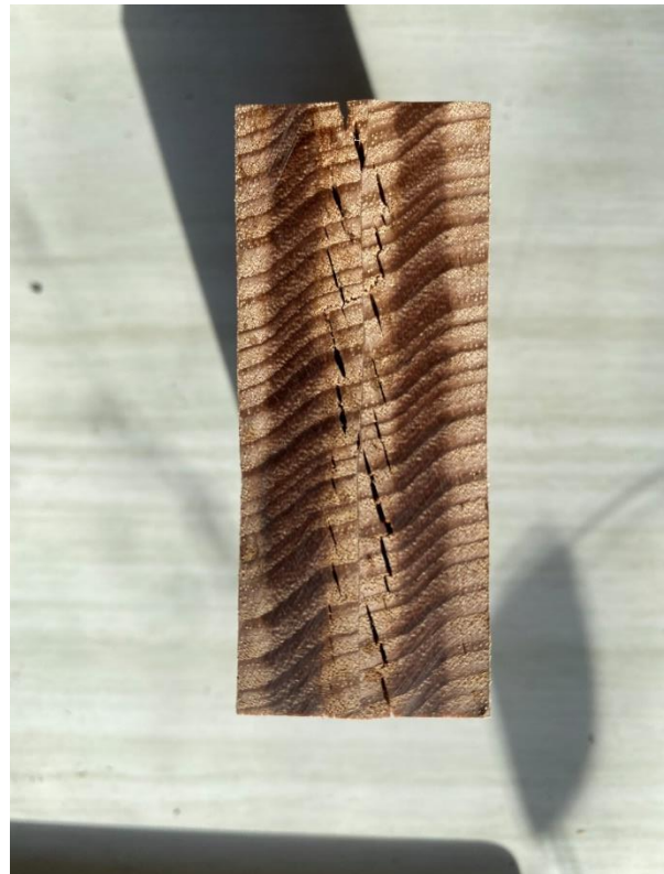
Figure 52. Eucalyptus delegatensis sample following the delamination test (Compression ratio: 37%; pressing temperature: 150°C; pressing time: 10 min; total delamination: 13.0%). Photo: Benoit Belleville.
