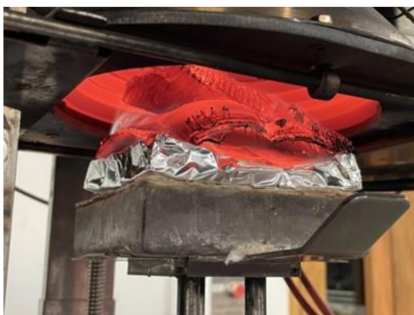
Figure 59. Interior fire-retardant treated sample being tested in cone-calorimeter, back wrapped in foil. Photo: Wenxuan Wu.
