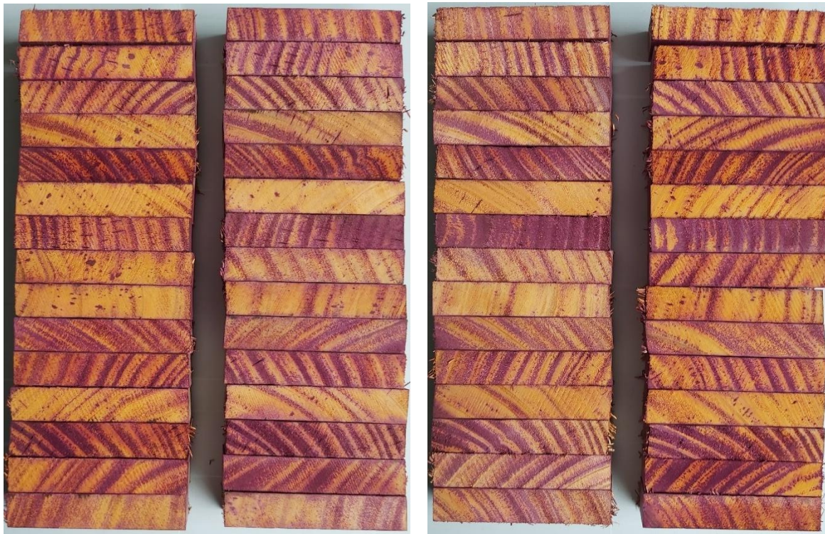
Figure 12. Penetration images of treated shining gum from charge 3+ACQ+adjuvants, left to right, showing copper penetration of ACQ, ACQ + B, ACQ + S and ACQ + V. Photo: Stuart Meldrum.
