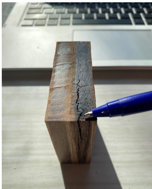
Figure 54. Eucalyptus regnans sample following the delamination test (Compression ratio: 37%; pressing temperature: 175°C; pressing time: 20 min; total delamination 5.8%). Photo: Benoit Belleville.
