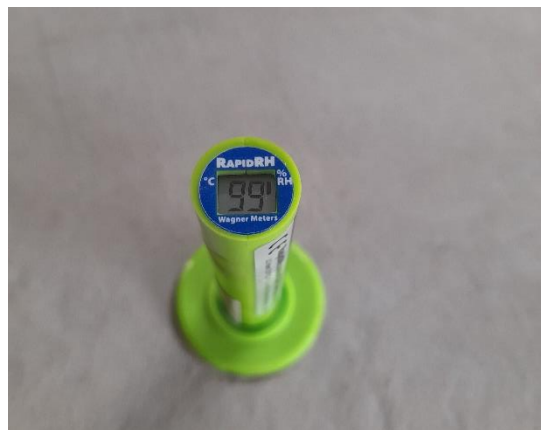
Figure 26: Builder measurement of slab condition
