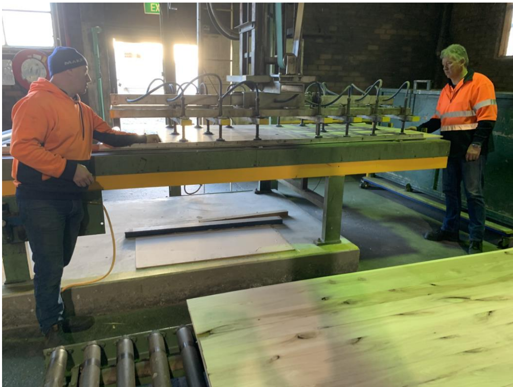
Figure 12: Post glue curing for fibre managed concept- PVA glue (water resistant) was subjected to hot pressing, all concepts showed good adhesion.
