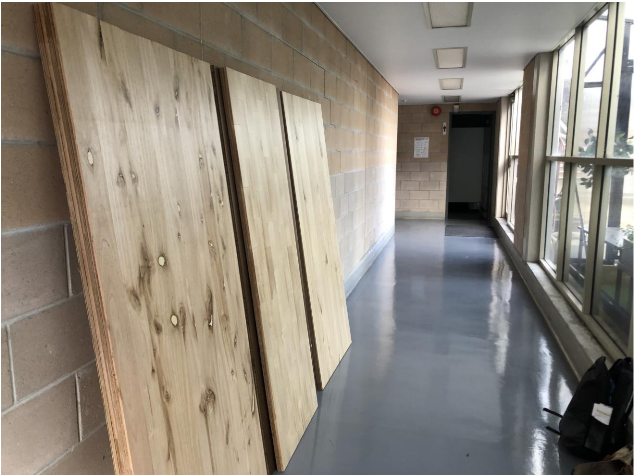
Figure 19: Panels with clear sealant (Urethane two-pack polyurethane waterborne coating system with a satin finish adhering to general industry practice) prepared for installation at LC college.
