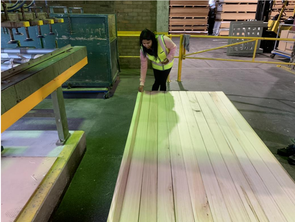
Figure 13: Post glue curing for sawlog managed concept: gaps were kept between each top layer board through the gluing process to plywoods to facilitate the ripping of panels.
