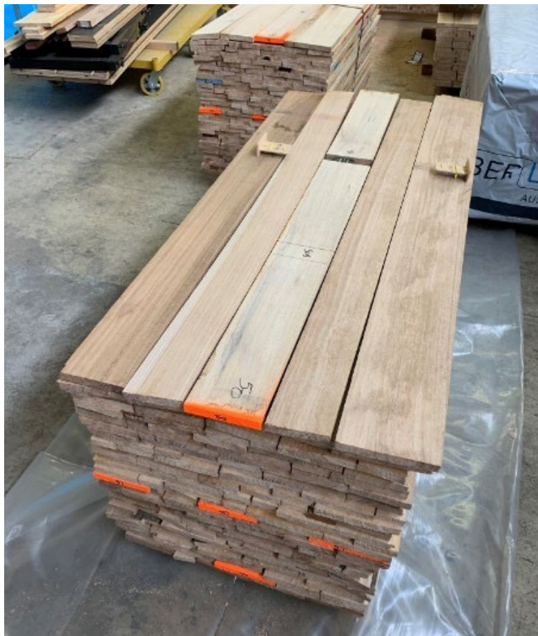
Figure 1: Timber pack with sensors and chosen sample boards. Orange paint highlights sample boards; top middle, west, middle, east and bottom middle.
