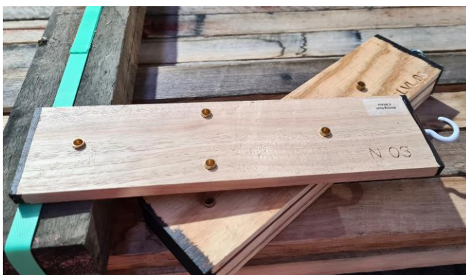
Figure 3: Pins fixed to the labelled sample's face.
