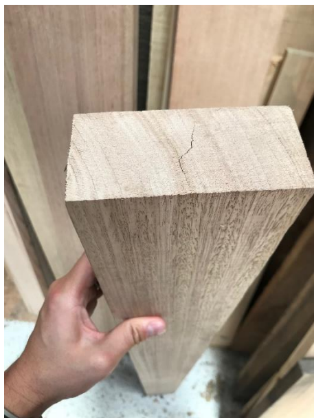
Figure 1: Board with MC-induced end splits
