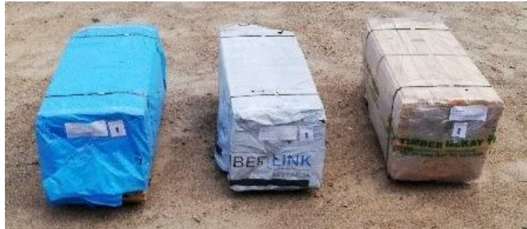
Figure 16: Three types of wrapping trailed in this sub-program. Poorly wrapped (left), fully wrapped - opaque (middle) and fully wrapped clear (right).
