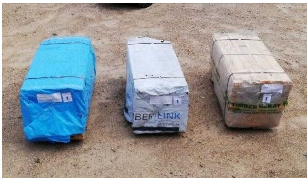
Figure 3: Three types of wrapping trailed in this sub-program. Poorly wrapped (left), fully wrapped - opaque (middle) and fully wrapped clear (right).
