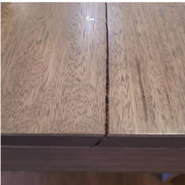
Figure 7: Splitting across a tabletop at a gum vein,
