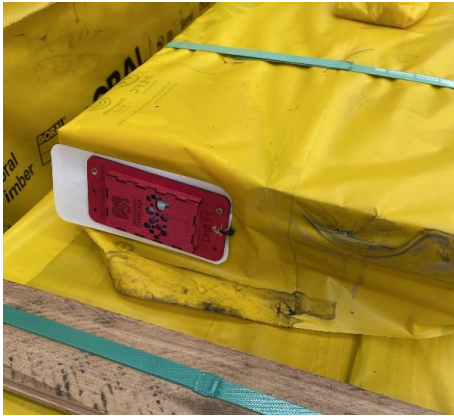
Figure 14: Mobile unit pack with temperature and humidity sensor ready for transport.
