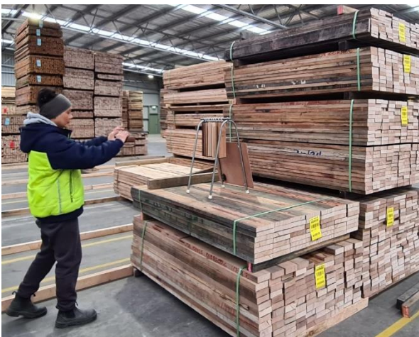
Figure 7: Static sensor and sample unit at a dry mill Bridgewater.
