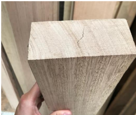
Board with MC-induced end splits
