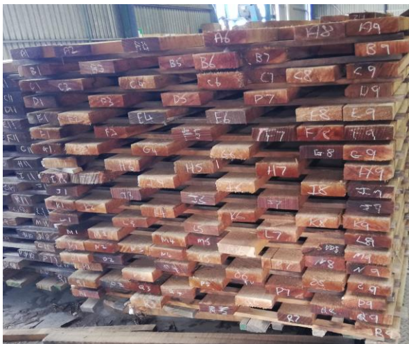
Figure 4: Board numbering in preparation for rack breakdown and data collection
