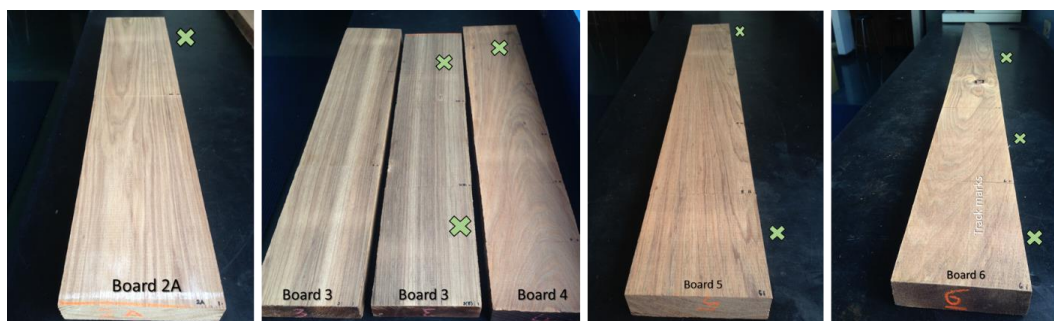
Figure 22: Pale sticker marks on Blackwood boards. Samples were shaved from sticker mark and face regions
