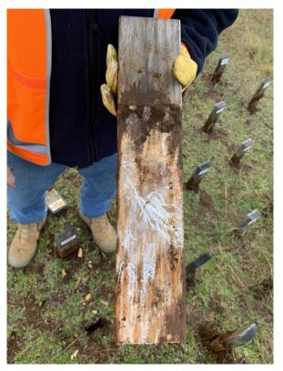
**Figure 3.** Mycelial growth on an in-ground stake at Upper Castra, Tasmania. Photo: Kyra Wood.
