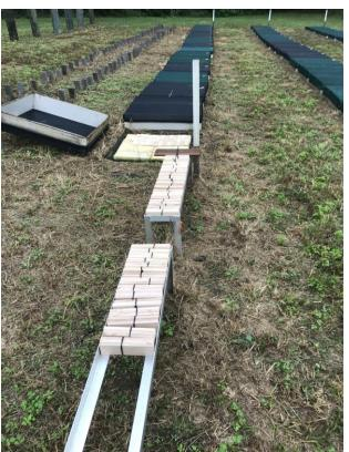
**Figure 12.** Thermo-mechanical densified material in sandwich arrays at Nambour, Queensland. Photo: Jeffrey Morrell.
