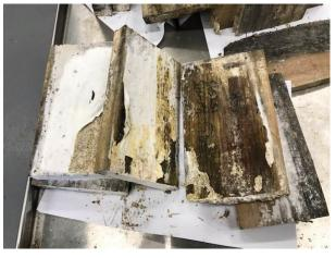
**Figure 41.** Example of ACQ treated blocks covered with an extensive mycelial mat and showing evidence of darkening and surface cracking at the end of the incubation period. Photo: Jeffrey Morrell.
