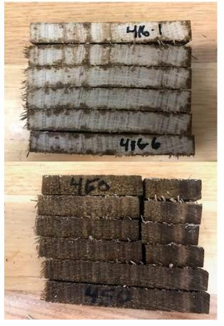
**Figure 32.** Examples of the sequential 20 mm thick cross cuts from 12 mm thick ACQ treated shining gum samples after the final wetting cycle showing minimal wetting on the upper sample and complete soaking on the lower one. Note the lower, wetted sample also experienced more deformation and cracking. Photo: Jeffrey Morrell.
