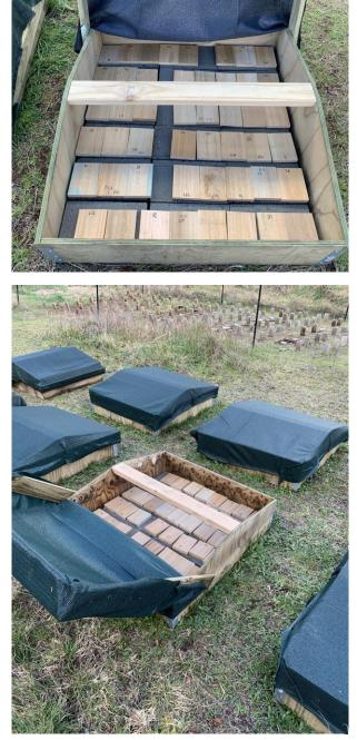
**Figure 10.** (Top and Bottom) Densified material, and MCA, ACQ, LOSP, and Kop-Coat treated material in ground proximity arrays at Upper Castra, Tasmania. Photo: Kyra Wood.
