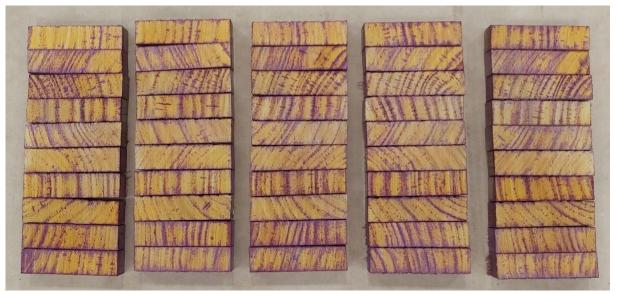
**Figure 27.** Example of 'candy-striping' effect in ACQ treated shining gum sprayed with a PAN indicator spray. Photo: Stuart Meldrum.
