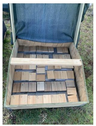
**Figure 9.** ACQ treated material of varying thicknesses in ground proximity array at Upper Castra, Tasmania. Photo: Kyra Wood.
