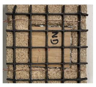
**Figure 33.** Example of grid used to restrain the compressed samples during cone calorimeter testing. Photo: Wenxuan Wu.
