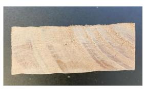
**Figure 21.** Example of internal collapse in 35 mm thick shining gum boards, several months after SCF impregnation. Photo: Kyra Wood.
