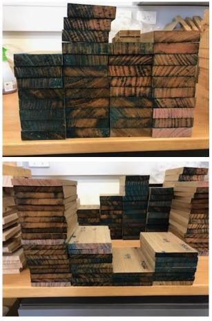
**Figure 28**. Examples of cross sections of ACQ treated *E. nitens* and *E. obliqua* samples of varying thicknesses showing the differences in degree of preservative penetration for 12 mm (bottom) and 25 mm (top) thick samples. Photo: Jeffrey Morrell.
