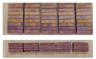
**Figure 19.** Tasmanian oak cross sections from boards VPI treated with ACQ, and sprayed with PAN indicator spray, charges 1 – 5 from left to right. 25 mm thick boards (top) and 5 mm thick boards (bottom). Photos: Stuart Meldrum.
