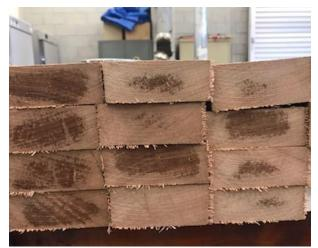
**Figure 26.** Solid piled boron treated *F. brayleyana* with substantial moisture still evident in the core of the boards after a twelve week diffusion period. Photo: Jeffrey Morrell.
