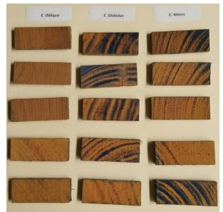
**Figure 16.** *E. obliqua, E. globulus, E. nitens,* (left to right) Charge 2 (matching boards in Figure 15 above) board cross sections treated with ACQ and sprayed with chrome azurol S, showing less penetration than with PAN indicator spray. Photo: Stuart Meldrum.
