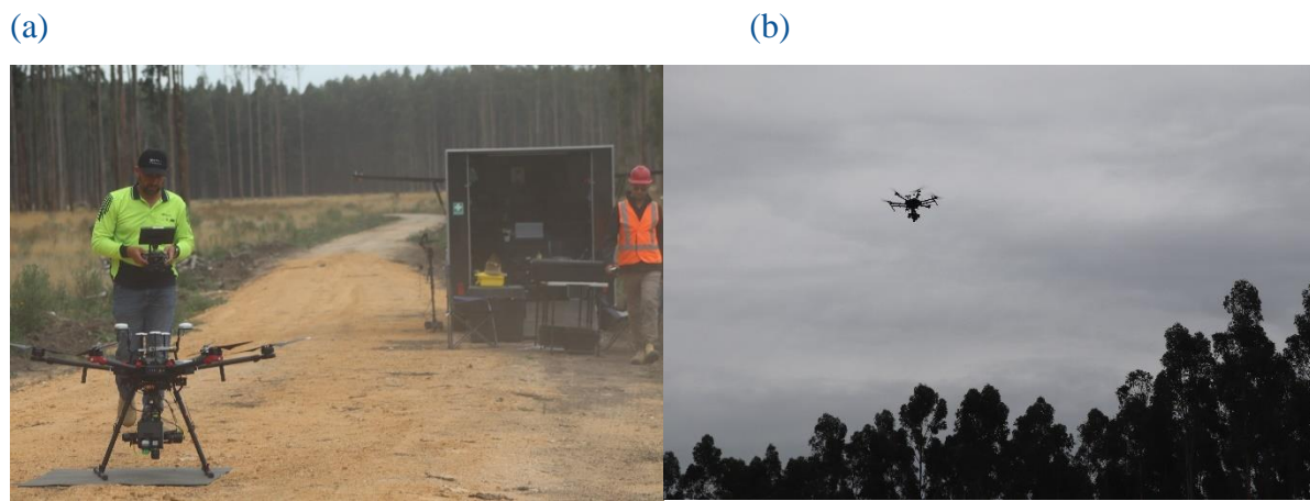
Figure 3: (a) Preparing DJI Matrice 600 for flight and (b) in flight over blue gum plantations.
