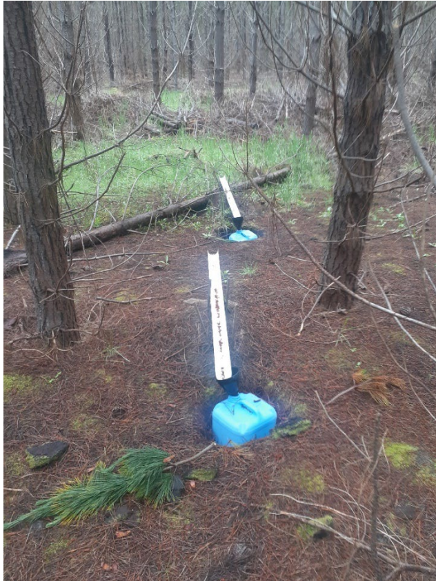
Figure 1: A photograph of throughfall collectors installed at a Pinus Radiata monitoring site
