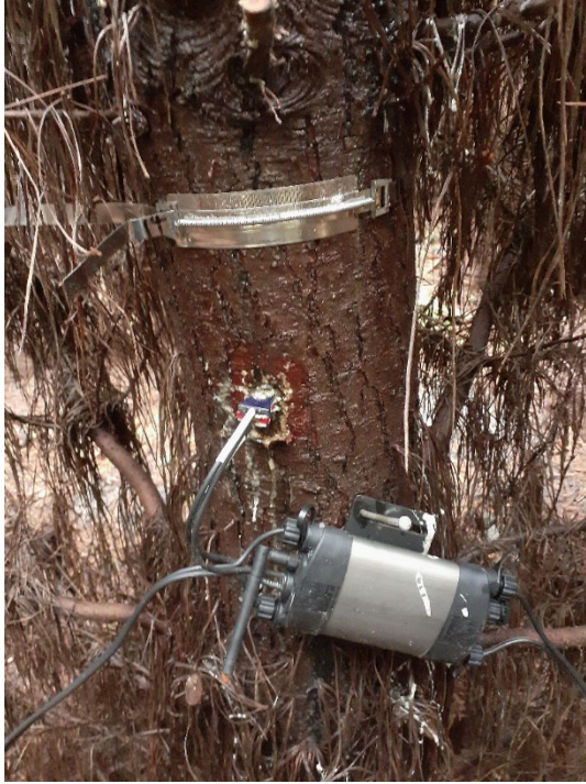
Figure 2: Photograph of a banded dendrometer on a pine tree which is also fitted with a sap flow sensor
