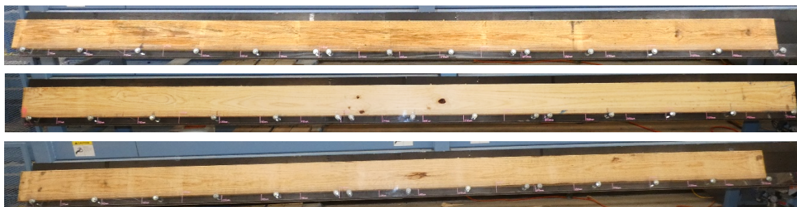
Figure 3.22 – No failure in tension test on high strength test pieces that exceeded the machine load capacity
