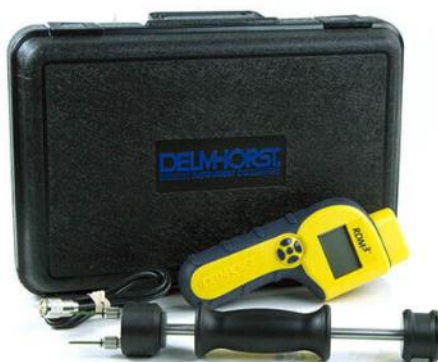
Figure 3.6 – Photo of the electrical resistance meter(model: Delmhorst RDM-3, serial 15104)
