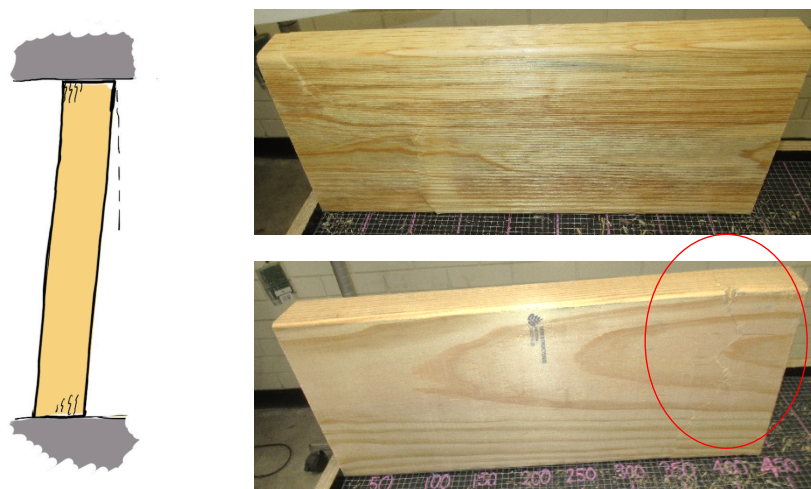
Figure 3.28 – Compression test failure by rotation of specimen
