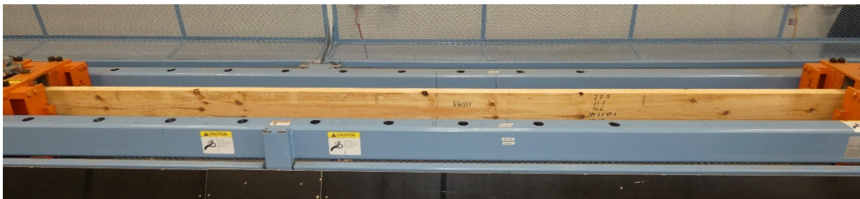
Figure 3.18 – Test set-up for measuring the tension strength parallel to grain (190x45 mm specimen)
