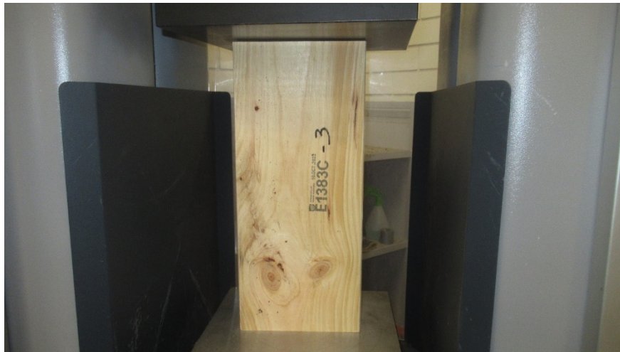
Figure 3.24 – Test setup for measuring compression strength parallel to grain (190x45 mm specimen)
