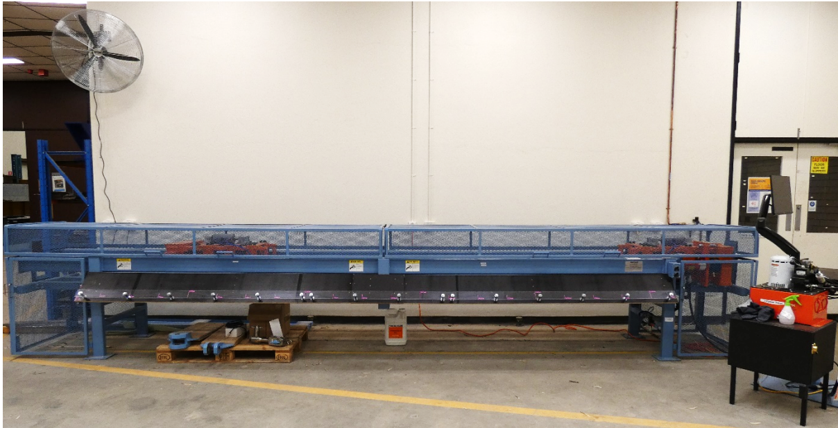
Figure 3.1 – Photo of the tension testing machine (Metriguard Tension Proof Tester, Model 403)
