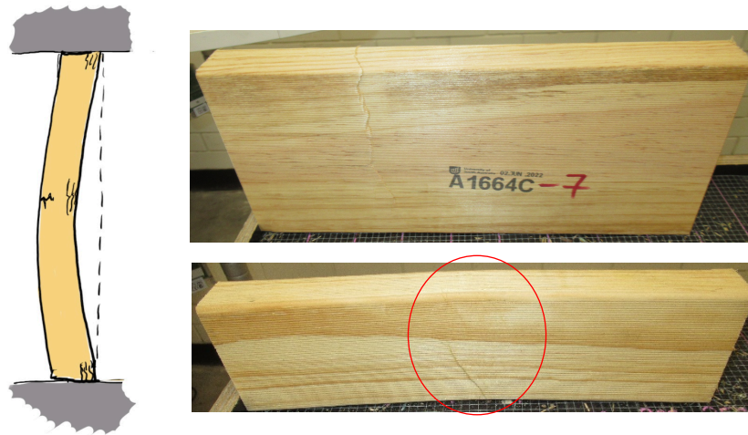
Figure 3.29 – Compression test failure by buckling or flexural failure of the specimen
