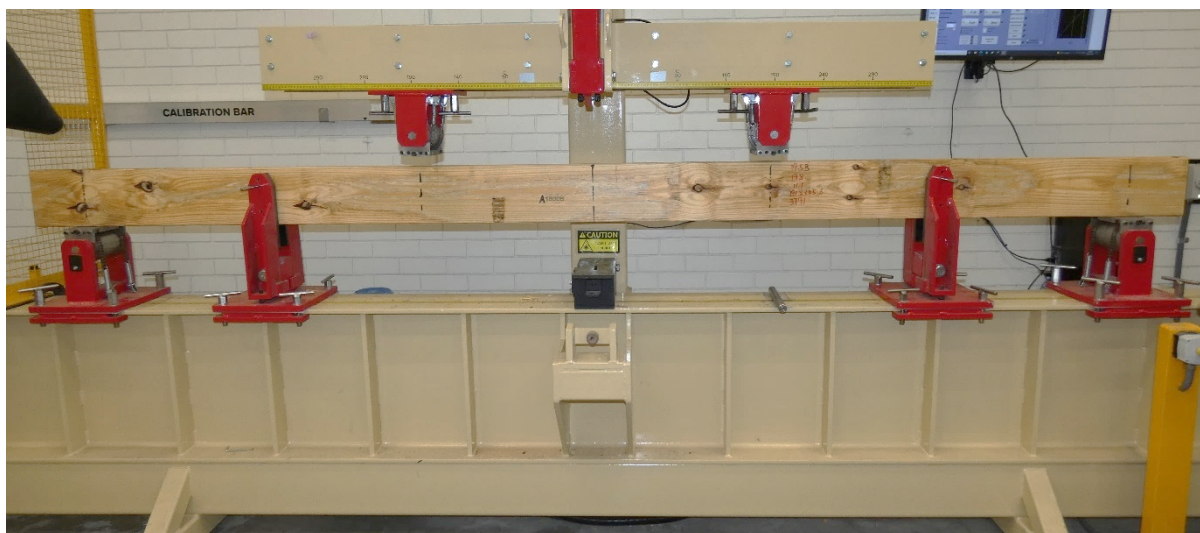
Figure 3.10 – Test set-up for measuring the apparent modulus of elasticity and the bending strength (190x45 mm specimen)
