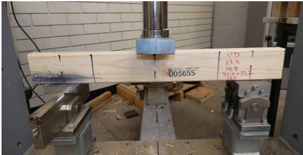
Figure 3.30 – Test setup for measuring shear strength (90x35 specimen)
