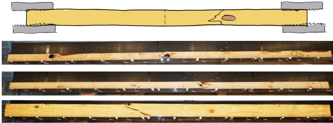
Figure 3.20 – Tension failure through knot or hole
