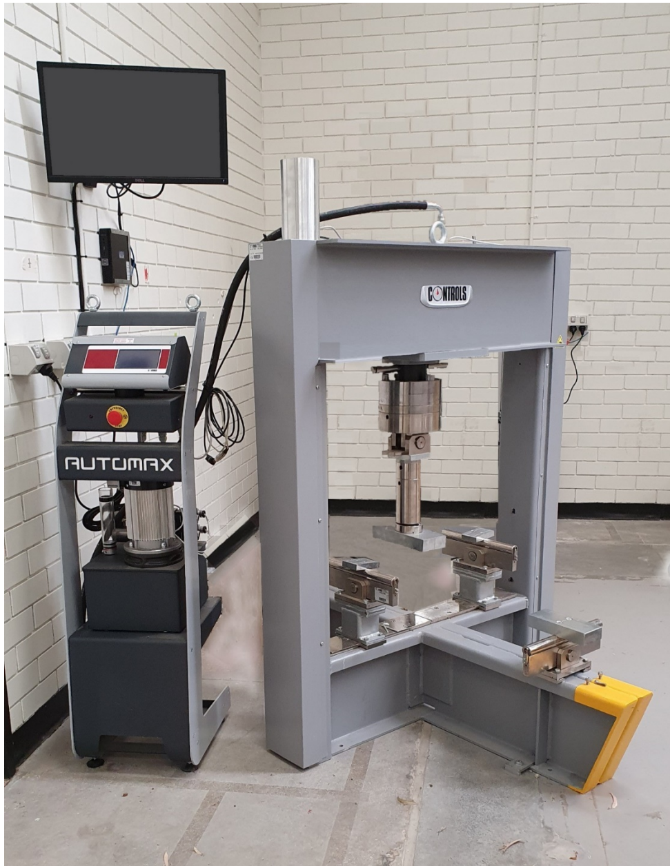
Figure 3.3 – Photo of the shear testing machine (CONTROLS Flexure Tester, Model AUTOMAX SMART-Line)
