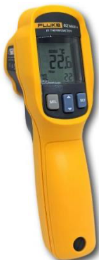
Figure 3.8 – Photo of the thermometer (model: FLUKE-62-MAX)
