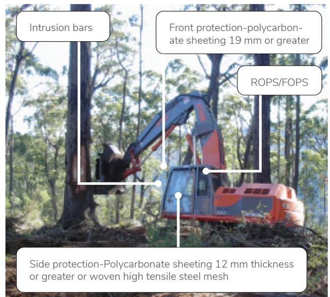
**Figure 3:** Mechanical harvester – excavator modified
