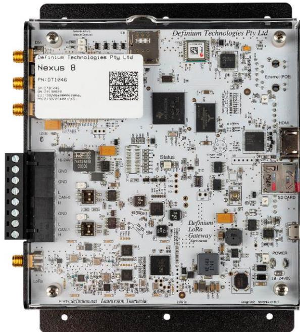
Figure 7: A Definium Nexus 8 LTE enabled LoRa gateway.
