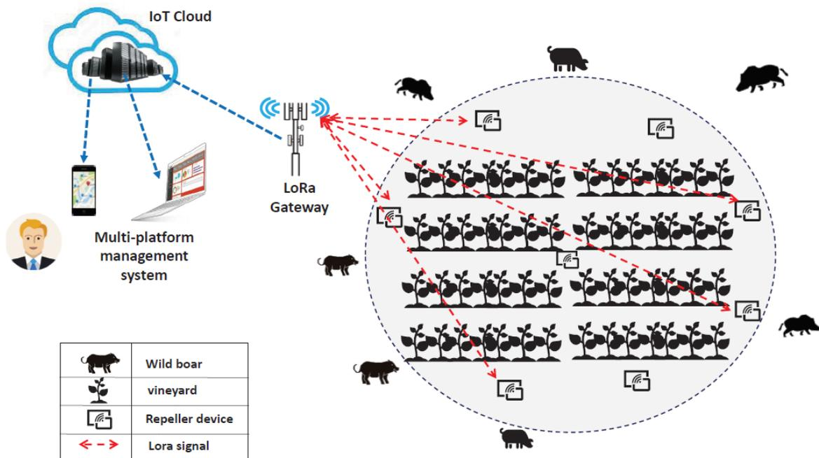
Figure 3: A schematic of an IoT system to monitor and manage wild animals (in this case wild boars in vineyards) from Ojo et al. 2021.
