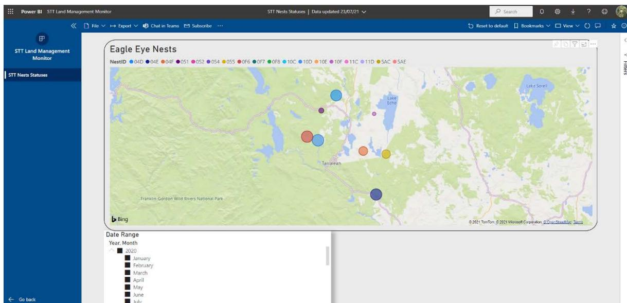
Figure 19: A MS Power BI report of the PIR readings for each nest are shown on a map as colored circles. The bigger the circle, the greater the level of activity detected.
