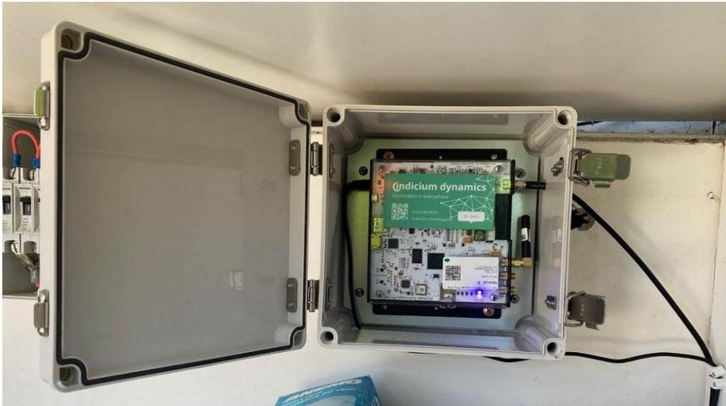
Figure 15: A Gateway installed on a fire tower and powered from 240 volts via a transformer.
