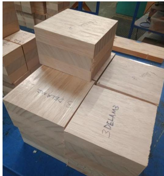
Figure 5. CLT cut into blocks for shear test.
