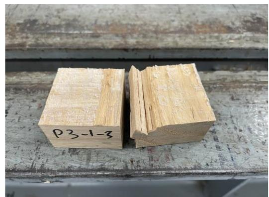
Figure 12. Samples showing bond line failure after block shear test.
