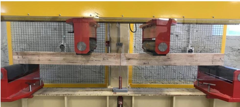
**Figure 1: Four-point bending test setup (Sample ref. A-1)**
