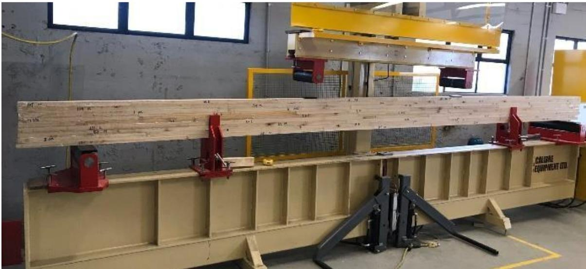
**Figure 2: Bending test of a combined glulam sample**
