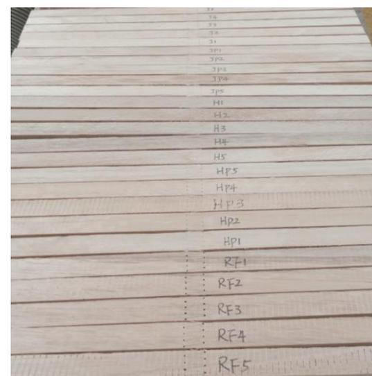
Figure 6. Finger joints with different glues
