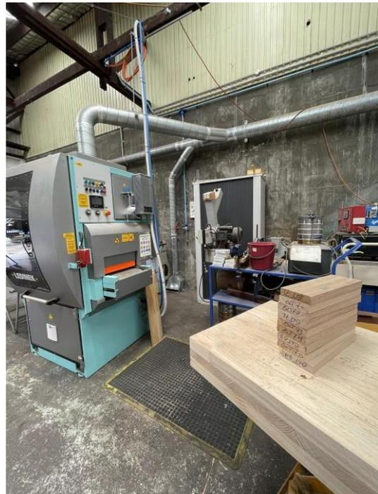
Figure 3. Face milling equipment at the DAF research facility, with some of our *E. nitens* sample boards waiting to be milled.
