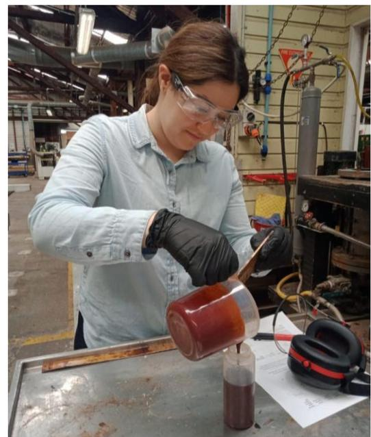
Figure 2. Azin mixing RF glue for the sample production at DAF research facility.
