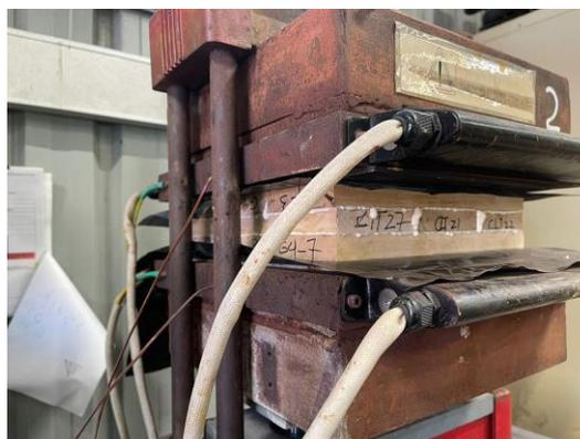
Figure 8. CLT parent billets in the press.
