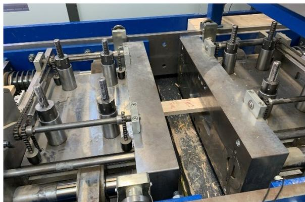
Figure 2: Specimen in the tension testing machine
