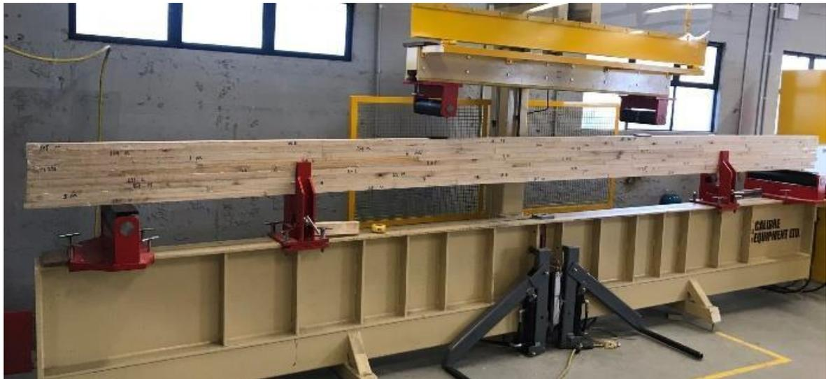
**Figure 5. Elevation view of the tested beam (a), Bending test of a combined glulam sample (b)**
