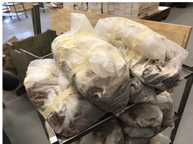
**Figure 39.** Plastic bags used to inoculate the samples in moist vermiculite for six months. Photo: Jeffrey Morrell.
