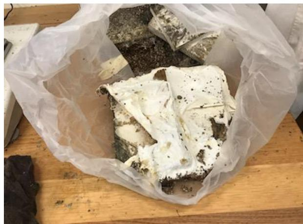
**Figure 40.** Examples of samples covered in thick mycelial mat in a freshly opened bag. Photo: Jeffrey Morrell.
