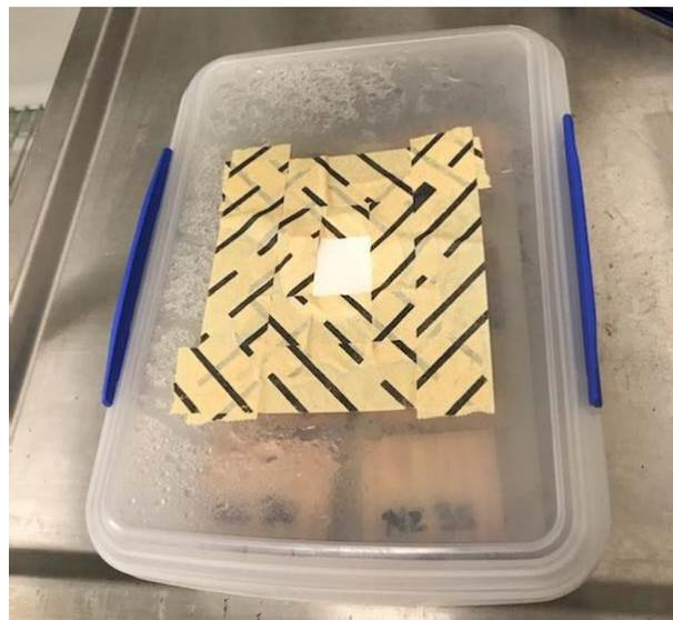
**Figure 32.** Agar block test using densified material.
