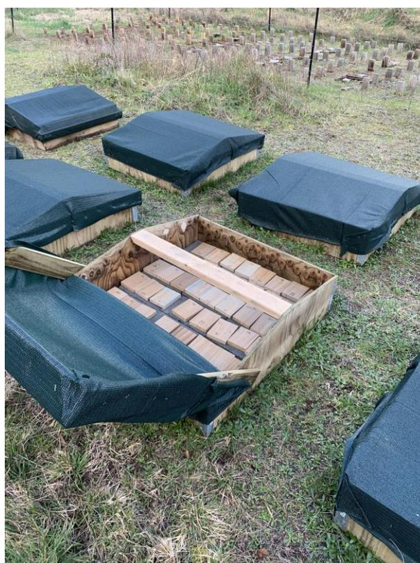
**Figure 10.** (Top and Bottom) Densified material, and MCA, ACQ, LOSP, and Kop-Coat treated material in ground proximity arrays at Upper Castra, Tasmania. Photo: Kyra Wood.
