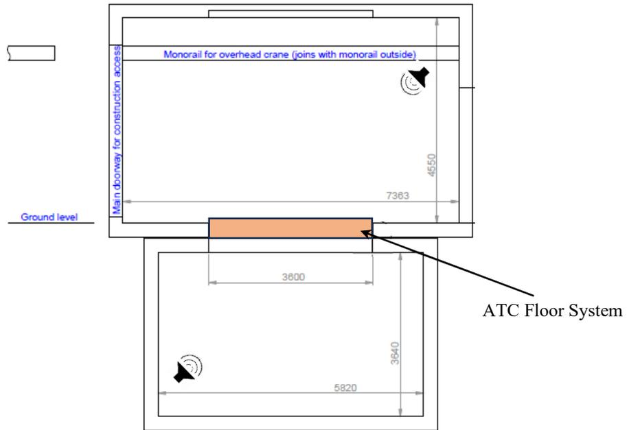
**Figure 16 – Section: CSIRO Acoustic Testing Facility**
