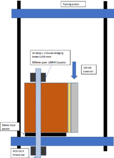
**Figure 5 – Shear Connector Test Set-up**
