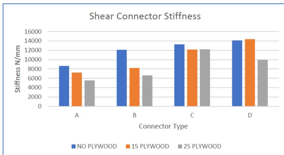
**Figure 9 – Mean Shear Connector Type Stiffness**
