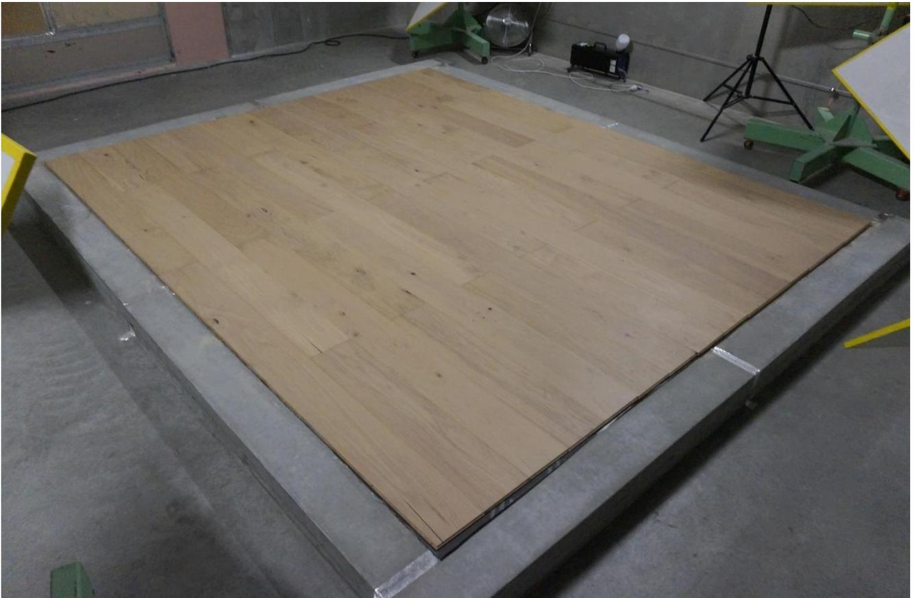
Engineered timber floating floor on top of ATC Composite Panel (as tested)
