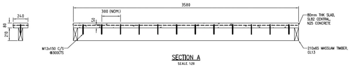
**Figure 10 – Structural Beam Test Section**
