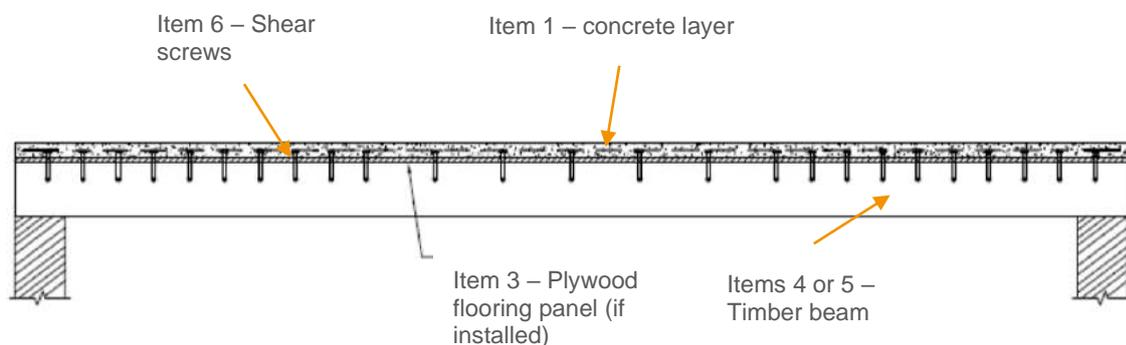
**Figure 1** Details of proposed floor systems
