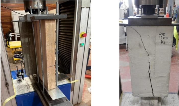
**Figure 6 – Shear Connector Test**
