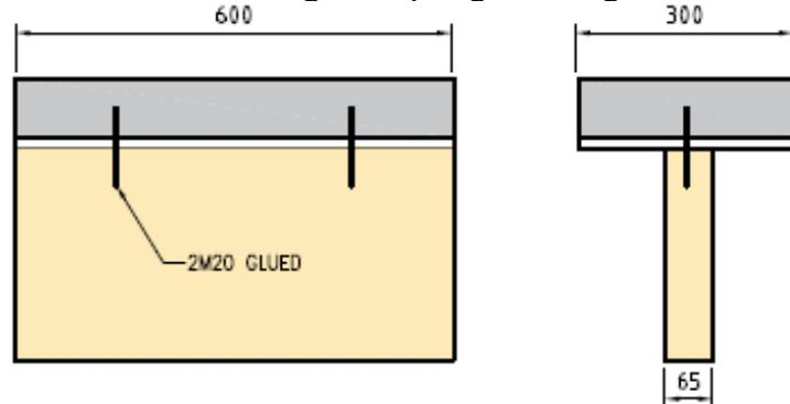
Individual 300 mm wide x (approx.) 400 mm deep x 600 mm long ‘T’ section test specimens, with a concrete slab 60 mm thick, were fabricated using each of these shear connector types with the following interlayers (refer Figure 4):
