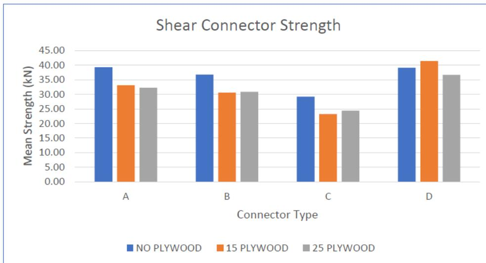
**Figure 8 – Mean Shear Connector Type Strength**
